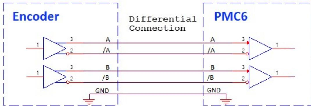
Note : Encoder GND should short to PMC6 GND.
