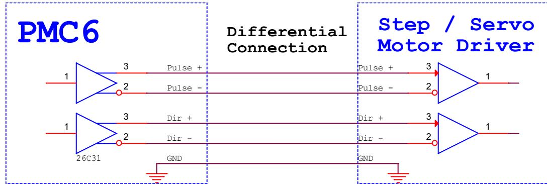
Note : Motor Servo GND should short to PMC6 GND.
