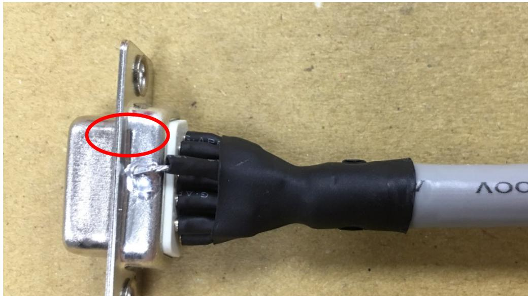
The cover of D-SUB is recommended in metal material.
